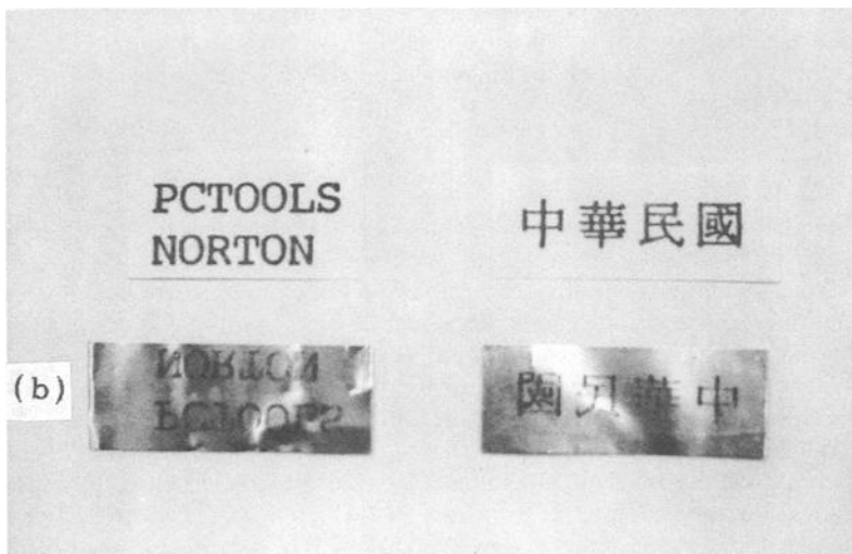
FIG. 1—Portions of the toner on the photocopies, (a) have been removed with the foil, (b).
